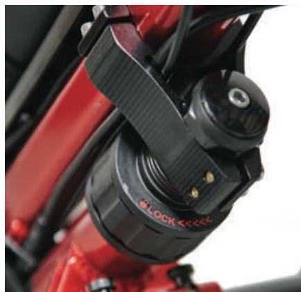
Locking headset for easier transfer & storage
