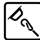
Figure 179. Sticker showing the location of the tie-down eyes.
