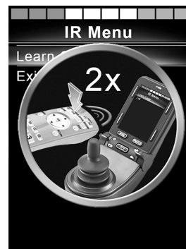
Figure 94. Point the remote control at the IR receiver. Press the button twice.
