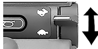
Figure 86. In mode Bluetooth® the right paddle switch is used to scroll up or down.
