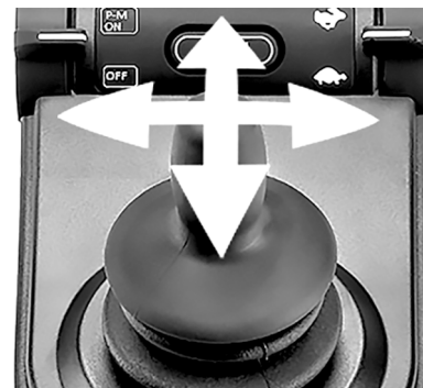
Figure 87. With the use of Bluetooth® the joystick can take control of the mouse functions.
