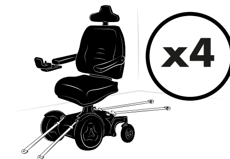
Figure 180. The wheelchair has four tie-down points. The wheelchair and tie-down position in this picture is generic.
